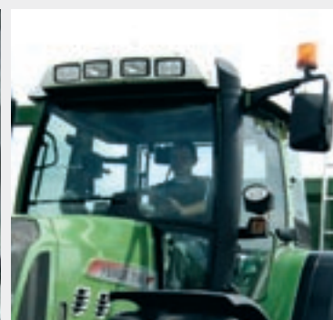
Auxiliary lighting with Xenon work lights; rotating beacon
