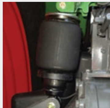
Pneumatic cab suspension
